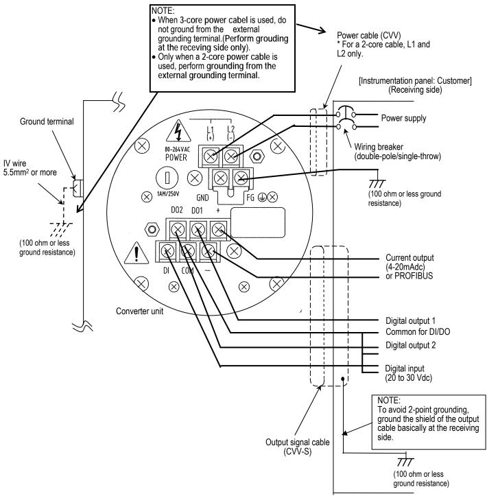
Figure 5.1 External Wiring Schematic Diagram
